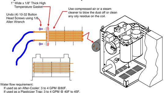
Note: To clean the cooling coil, use compressed air or a steam cleaner to blow the dust off or clean any oily residue on the coil.
